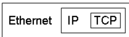
Figure 7. TCP packet embedded inside an IP packet, embedded in an Ethernet frame
